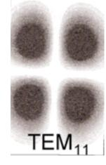
Larger gain due to larger volume, higher diffraction losses
