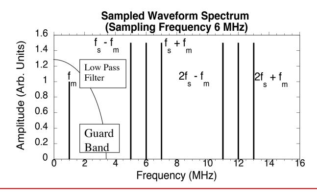
In the example above the 'information signal' is simply a single tone at a frequency  $f_m = 1 \text{ MHz}$  - ironically this standard example uses the archetypal 'no information' signal. The sampling frequency is 6 MHz or 6 Samples/ Cycle.
