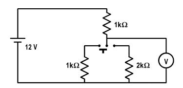
The slide switch is a make-before-break type When the switch changes over, the output voltage indicated by the voltmeter goes from:
