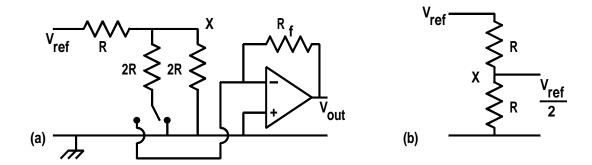
Most commonly used system is called the R-2R ladder converter.
