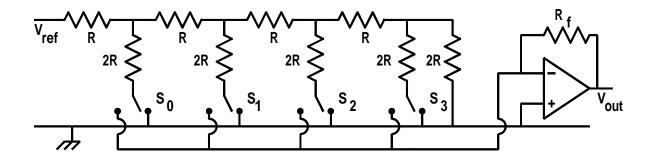
The current to voltage circuit sums all of the currents through the 2R resistors from each of the voltage tap off points on the R-2R ladder and gives an output voltage
