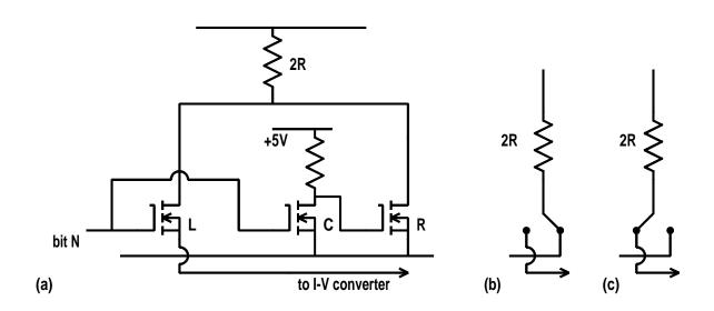
FET switches are used with R-2R ladder network.
