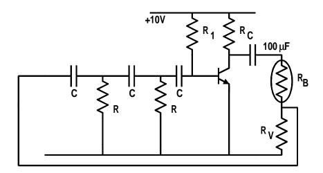
Amplitude stabilization by control of feedback.
