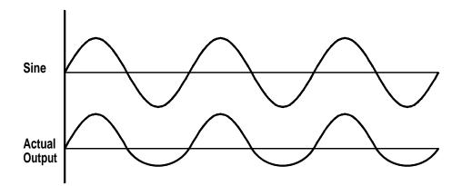
Distortion due to saturation nonlinearity.
