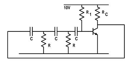
Positive feedback causes the circuit to go into oscillation.
