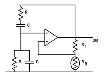
Frequency control with a twin ganged potentiometer for the two Wein bridge resistors. Decade changes of frequency are obtained by switching in pairs of capacitors
