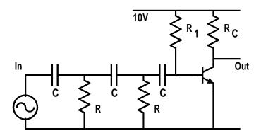
Phase shift network and amplifier. A sinusoidal signal applied to the input is phase shifted and attenuated in each of the three CR filters.
