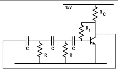
Design a transistor phase shift oscillator for a fixed frequency of 300Hz.
