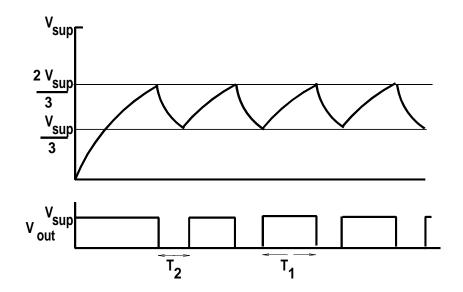
Capacitor and output voltage waveforms for the 555 Timer.
