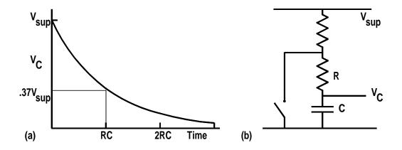
RC discharging curve. Close switch at t=0Set up differential equation
