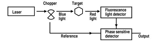
Laser beam is chopped at frequency  $F_R$  by a rotating chopper blade.
