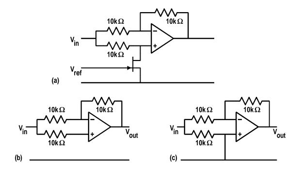
The circuit for the phase sensitive detector is therefore an amplifier which is switched between a gain of +1 and -1 by the application of the reference square wave.
