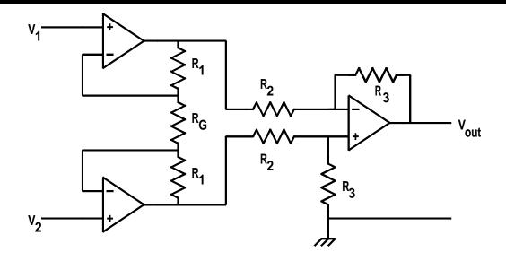
Consider the resistor chain  $R_1$ ,  $R_G$  and  $R_1$ . Voltage across the gain setting resistor,  $R_G$ , is  $V_1-V_2$
