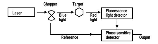
Chopper and phase sensitive detector configuration.
