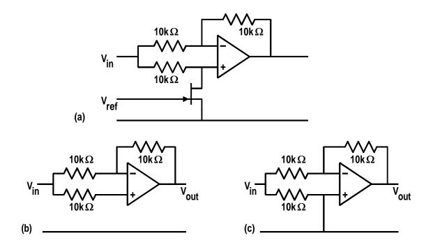
Basic phase sensitive detector circuit A reference square wave signal from 0V to -5V is available from the chopper Reference is synchronized with the signal to be detected. This signal is applied to the gate of the FET.
