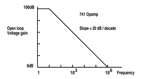
Gain is  $A=1+\frac{5000}{100}=51$  or 34dB. Plot the 34dB line and the bandwidth is obtained to be about 30kHz. The thermal noise from the  $500k\Omega$  resistor is given by
