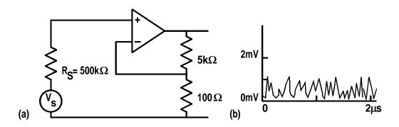
Calculate the thermal noise from the  $500k\Omega$  resistor at  $20^oC$  which would be observed on an oscilloscope connected to the output of the circuit
