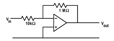
Inverting amplifier which has a gain of
