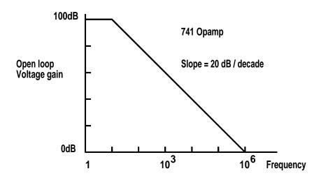
Open loop gain as a function of frequency for the 741.
