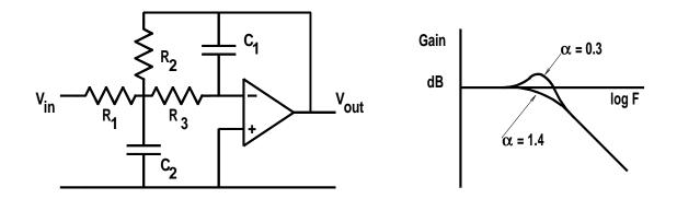
Estimate  $C_1$  and use the formulae for  $C_2$ ,  $R_1$ ,  $R_2$  and  $R_3$ .
