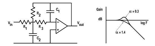
Design a low pass filter for a cutoff frequency of 1500Hz, a gain of 12 and 3dB of peaking at the band edge.
