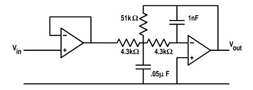
We do not know the signal source resistance, so it is good practice to isolate the filter from the signal source by using a voltage follower stage in the input which has a high input impedance and low output impedance.
