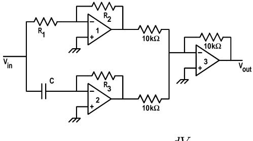
$$V_{out} = 3.3V_{in} + 2.2\frac{dV_{in}}{dt}$$
