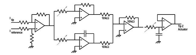
STM scanning tip height servo control Used to move the scanning tip up and down as it scans the surface in Burleigh Instruments Scanning Tunneling Microscope The input signal is the tip tunneling current. The output signal drives the tip in the z direction.
