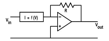
The forward function. Suppose we have a device in which the current through the device is related to the voltage across the device by some arbitrary function such as I = f(V).
