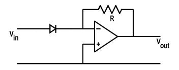
Derive an expression for the output voltage from this circuit
