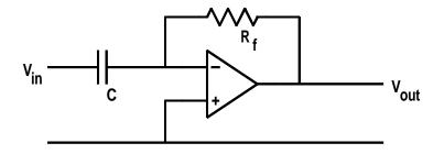
The output from a differentiator circuit is given by:
