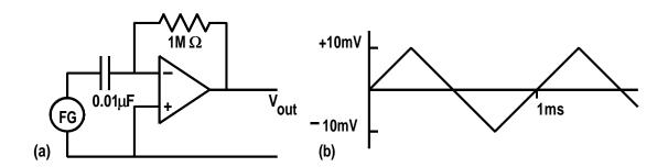
Function generator, FG, gives output triangular waveform of frequency 1kHz and amplitude 10mV
