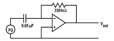
Calculate the output voltage waveform for an input triangular waveform of frequency 250 Hz and of amplitude 30 mV.
