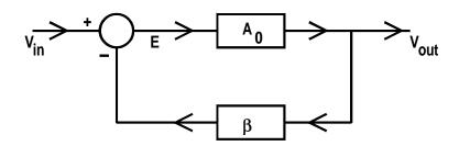
If a fraction,  $\beta$ , of the output of an amplifier is fed back and subtracted from the input to the amplifier and if the open loop gain of the amplifier is large, the closed loop gain of the amplifier is given by:—
