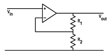
Analyse the noninverting amplifier shown in Figure 41.4 in terms of a negative feed back system.
