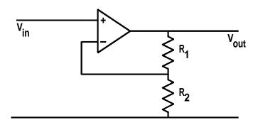
The gain of a noninverting amplifier is given by:—
