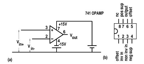
An op-amp has two inputs, an inverting input  $V_{in-}$  a noninverting input  $V_{in+}$ .
