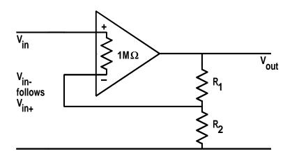
The op-amp has been designed to have an input resistance between the inverting and noninverting inputs of at least  $1M\Omega$ .
