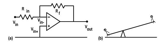
Inverting amplifier circuit and model
