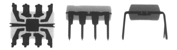
Fine wires connecting the silicon chip mounted on the lead frame to the pins of the dil package
