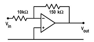
The gain of an inverting amplifier is given by:—
