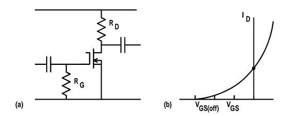
Basic MOSFET amplifier circuit and input characteristic
