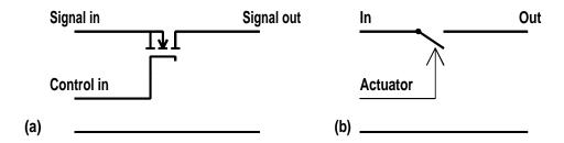
Control is isolated from the signal which is being switched.
