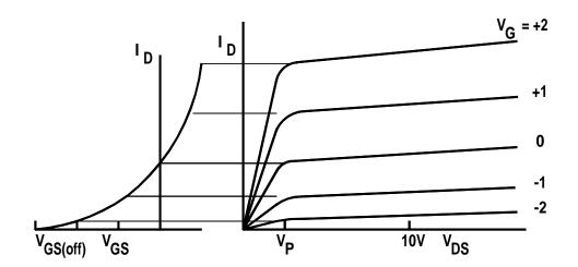
n channel depletion mode MOSFET Negative voltage applied to the gate, MOS-FET operates in depletion mode Positive gate voltage, the MOSFET operates in enhancement mode
