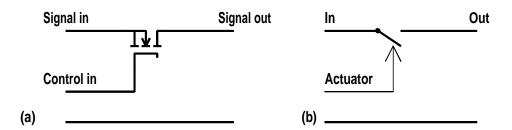
MOSFET analogue switch using an enhancement type MOSFET.
