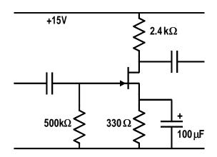
Calculate the component values and supply voltage to obtain a small signal voltage amplification,  $A_V=-6$  and an input impedance of  $500k\Omega$ .
