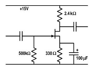
$R_G = 500k\Omega$  gives required input impedance
