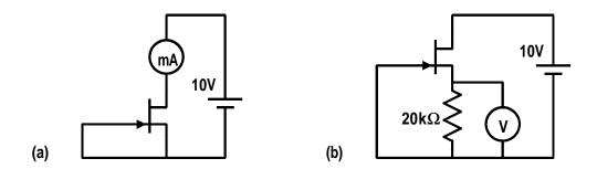
Circuits to measure  $I_{DSS}$  and  $V_{GS(off)}$  for a JFET
