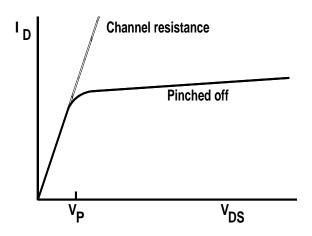
Effect of the pinch off mechanism Another mechanism operates.
