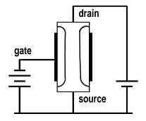
As the gate reverse bias is increased the depletion layer becomes thicker reducing the width of the conducting channel and therefore reducing the current flowing for a particular source to drain voltage
