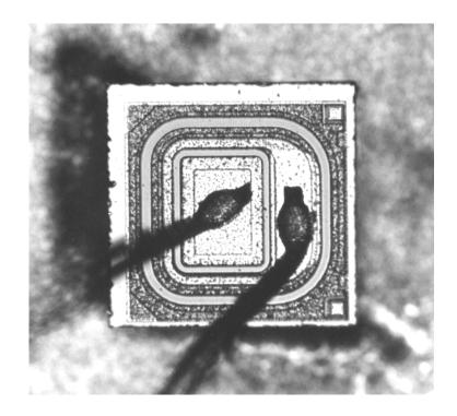
Microphotograph of a BC109 transistor
