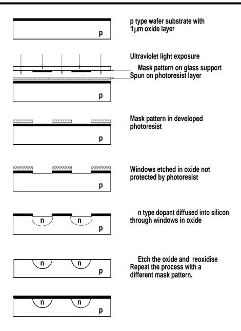
Photolithography using a negative photoresist
