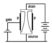
As the source to drain voltage is increased the depletion layer at the drain end of the channel becomes thicker due to the greater reverse bias at that end of the channel. This reduction of channel width tends to balance the greater current due to the greater voltage along the channel.
