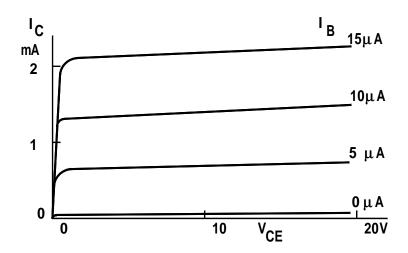
Characteristic curves have a small upward slope or large dynamic resistance 0.2mA for 20V in  $V_{CE}$  gives  $R_{DYN}=100k\Omega$  Current mirror shows a small dependence on the  $V_{CE}$ .
