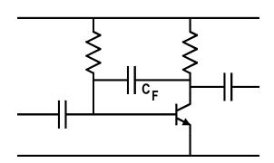
Use collector—base capacitance to reduce high frequency gain
