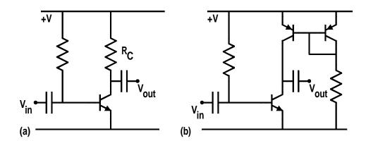
Use a pnp current mirror as instead of the collector resistor.
