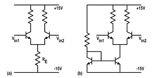
Current mirror used as emitter resistor in differential amplifier
