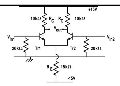
$v_{in}$  applied to one input only is equivalent to  $+\frac{v_{in}}{2}$  applied to one input and  $-\frac{v_{in}}{2}$  applied to the other input due to coupling action of the shared emitter resistor.
