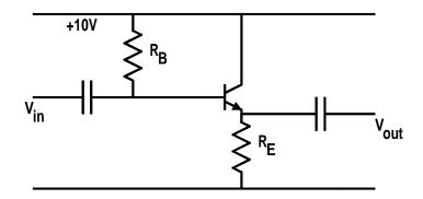
Emitter follower or common collector Signal applied at the base changes the base voltage.
