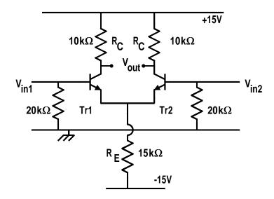
Positive voltage signal at base of left transistor gives more emitter current.
