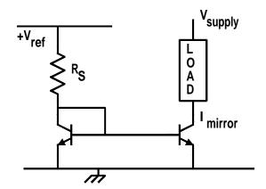
Left transistor is diode connected transistor Voltage drop across the emitter-base junction diode is for a current of  $\frac{V_{ref}-0.7}{R_S}$ .
