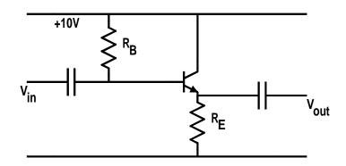
Input impedance of the emitter follower Input voltage  $v_{in}$  gives  $v_b$  which gives  $i_b$ . Current across the emitter base junction and in  $R_E$  is  $i_e=\beta i_b$ .
