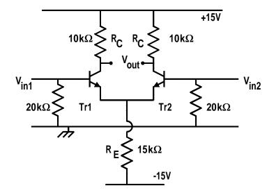
No input signals present current in  ${\cal R}_E$  divides equally between the two transistors Equal voltages at the two collectors and a differential output voltage between the two collectors of 0V.
