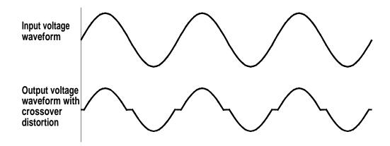
Minimise crossover distortion by providing some DC forward bias for the transistors even when when there is no input signal.
