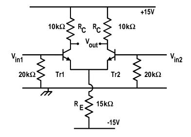
The circuit is symmetrical with a signal applied to the base of each transistor.
