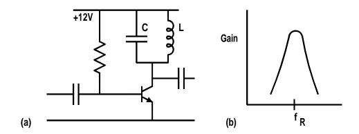
Tuned amplifier The gain of a common emitter amplifier is given by  $-R_C imes \frac{I_E}{25mV}$  which is essentially independent of frequency.
