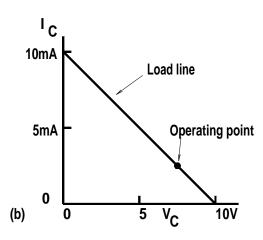
Transistor Load Line Unit 31, Example 1  $V_C = 7.7V$  and  $I_C = 2.3mA$  Modulate the base current in some way.
