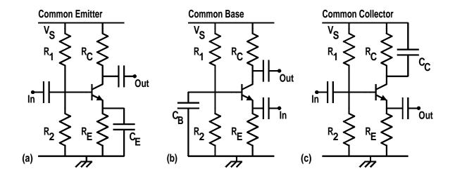
Common Collector Amplifier in (c)
