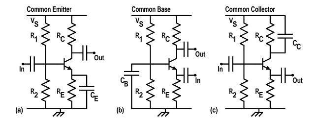
Common Emitter in (a) the emitter is grounded via the  $\mathcal{C}_E$  so the emitter voltage does not vary
