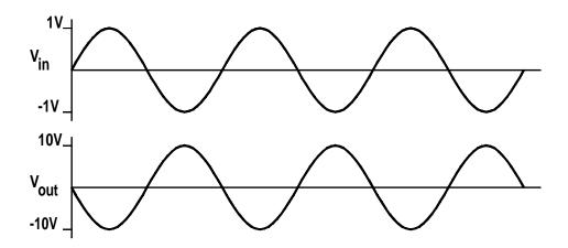
Oscilloscope trace of input and amplified signals for A=-10  $v_{out}$ , may be an inverted and amplified version of the input signal,  $v_{in}$
