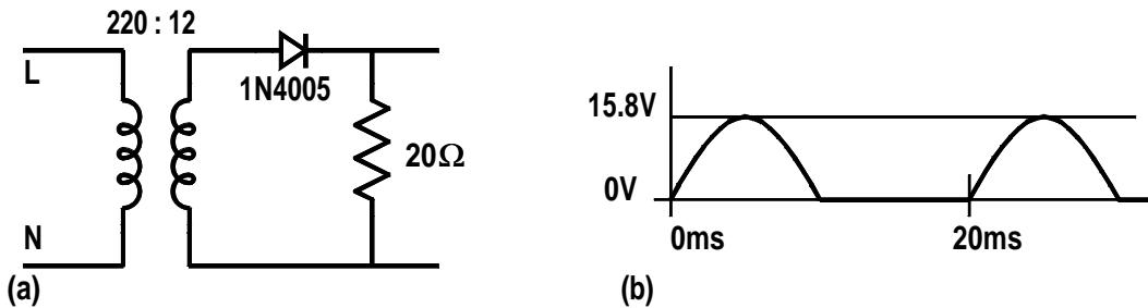
Output across load resistor  $R_L = 20\Omega$
