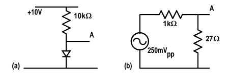
Effective circuit for the AC component of signal
