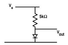
Calculate the change in the voltage across the diode if the setting of the power supply voltage,  $V_+$ , is changed from +10V to +11V.
