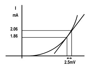
We first make the approximation that the DC voltage across the diode is 0.7V.
