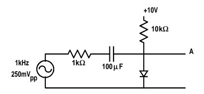
Calculate the output voltage waveform which would be observed on an oscilloscope connected to point A
