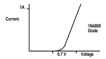
Usually the diode current is at least 1mA. From the diode characteristic curve, the expected value for the voltage across the diode is then close to the knee voltage for currents in the range from 1mA to about 100mA. This is called the "small signal region".
