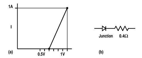
A 1N4005 type silicon diode passes 1.0A for a forward voltage of 1.1V. Sketch the diode characteristic and calculate the bulk resistance of the diode.
