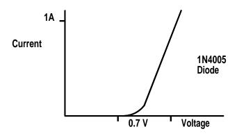
Measured I–V characteristic of a real silicon diode
