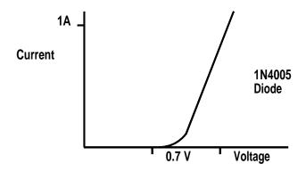
Measured I–V characteristic of a real silicon diode
