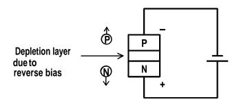
Junction diode in reverse bias Anode negative— Cathode positive.
