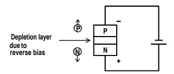
Even when the diode is reverse biased, a very small current flows.
