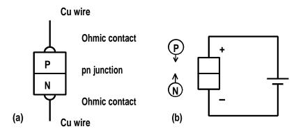
One fabrication problem relates to making a connection to the semiconductor material. If a metal, which is essentially an n type conductor, is connected to a p type semiconductor then, in principle, a pn junction is formed which would have some rectifying properties.
