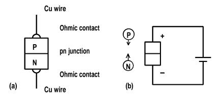
Diode construction and operation in forward bias.
