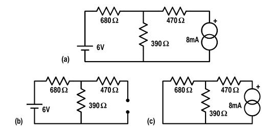
Calculate the current in the  $390\Omega$  resistor
