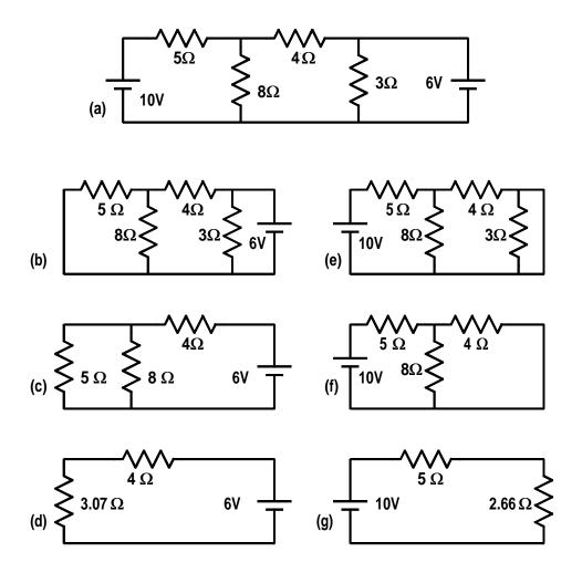
Calculate the current in the  $8\Omega$  resistor
