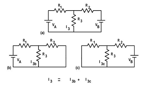
Split the x circuit before applying principle of superposition
