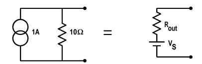
Convert from Norton to Thévenin equivalent circuit:— Calculate the Thévenin equivalent of the Norton circuit
