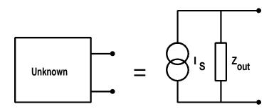
In order to measure the Norton equivalent of any circuit, it is only necessary to measure the open circuit voltage and the short circuit current.
