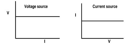
The characteristic curves for a voltage source and for a current source
