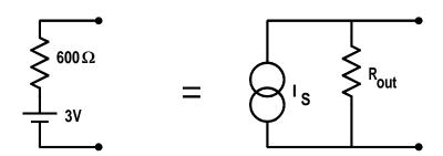
Calculate the Norton equivalent circuit Short circuit current.
