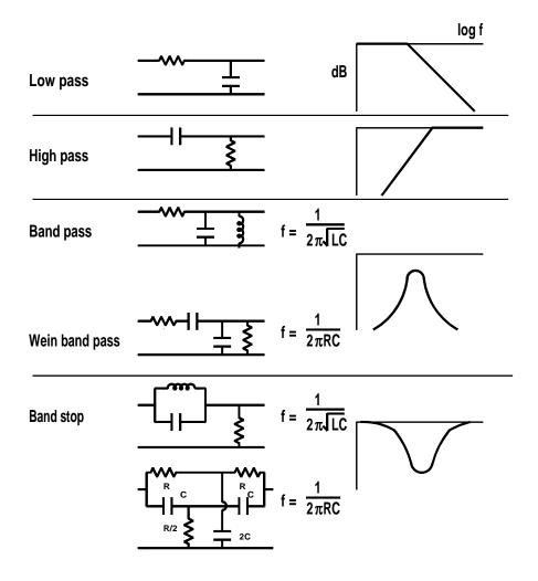
Typical filter circuits and response curves
