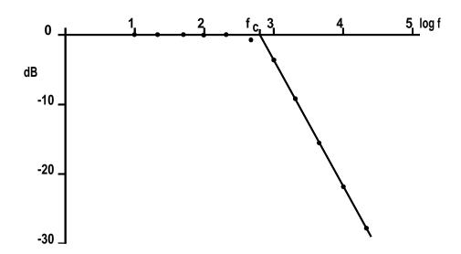
The response curve can be approximated by two straight lines through ( $\log f_c$ , 0dB).
