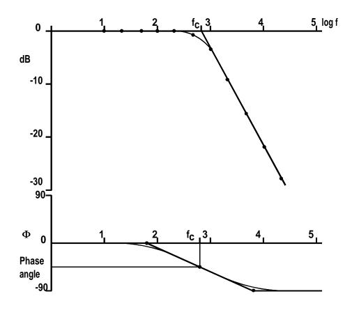
The RC circuit is a low pass circuit.
