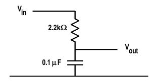
Calculate the frequency response by repeating the calculations of Example 15.1 for a range of frequencies.
