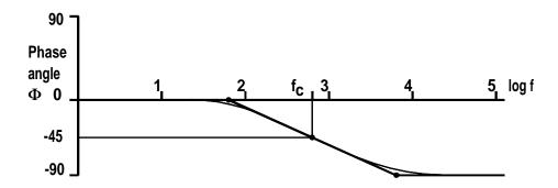
When the amplitude response and the phase response are combined on one diagram with the log frequency scale the pair of curves is called a Bode Plot.
