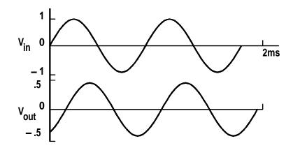
We calculated a phase shift of -1.12 radians. In the oscilloscope diagram the output waveform is displaced to the right by 1.12 radians or 64 degrees relative to the input voltage waveform.
