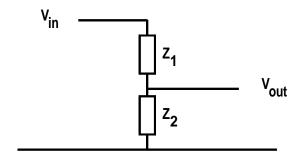
Replace the resistors of potential divider by any combination of resistors, capacitors or inductors in series or parallel.
