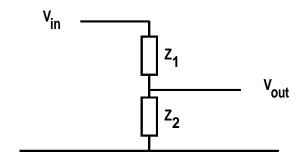
The ratio of output to input voltage is then
