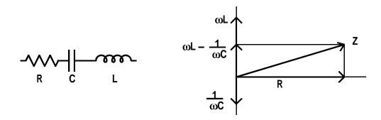
The resultant impedance, Z, of the three components connected in series is shown in the diagram.
