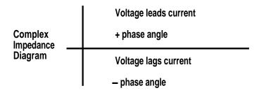
The current waveform is taken as the reference and the sign of the phase angle is + when the resultant impedance lies in the top half of the diagram and – when the resultant impedance lies in the bottom half of the diagram.
