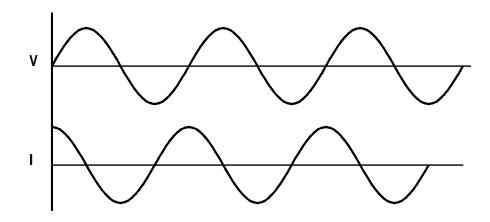
Apply a sinusoidal voltage waveform across a capacitor.
