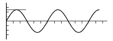
The maximum of the waveform is at 2.5 division and therefore the amplitude of the waveform is  $2.5 \times 2V = 5.0V$ .
