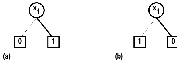
Figure 18.2: (a) Q = x_1 and (b) Q = \overline{x_1} . .
