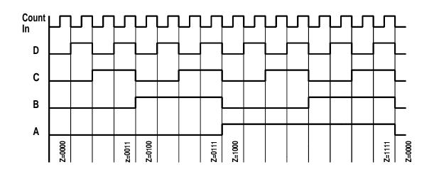
Waveform observed on a five channel oscilloscope for the four bit binary counter.
