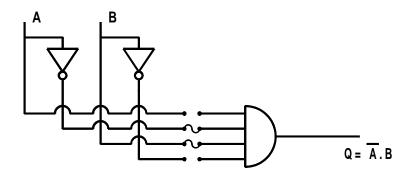
The same AND gate with two of the fuses burned out giving a logical output of  $Q = \overline{A}.B$ . The unconnected inputs to the AND gate default to logic 1.
