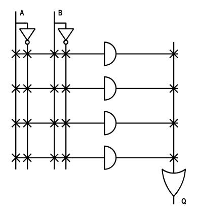
The same structure as that in Figure 21.3 but with the fusible links shown as  $\times$ .
