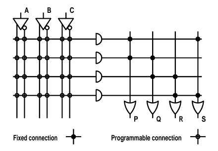
A Programmable Array Logic (PAL) configuration. These devices utilize CMOS technology and the links at the grid crossings are only formed when the device is programmed. The programmable links are shown with a circle. The manufactured-in fixed links are shown with a filled circle.
