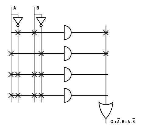
The reduced schematic for the XOR function  $Q = \overline{A}.B + A.\overline{B}.$
