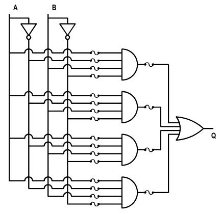
The structure which allows the implementation of any or all of the four canonical terms of the SOP formed from two inputs, A and B.
