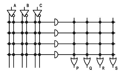
The Programmable Logic Array (PLA) configuration.
