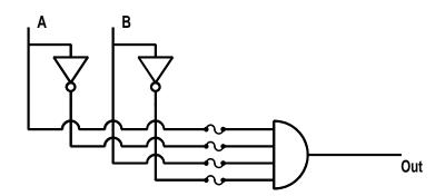
A 2 input system using a  $2 \times 2 = 4$  input AND gate with all possible input signals connected through fuses.
