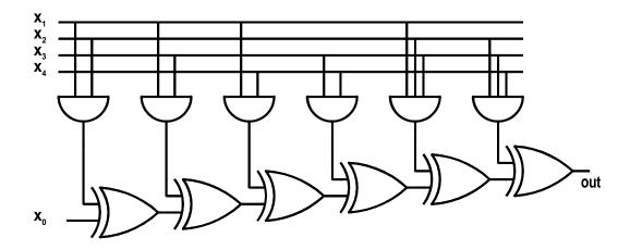
Test for faults on input lines connected to EVEN number of AND gates with
