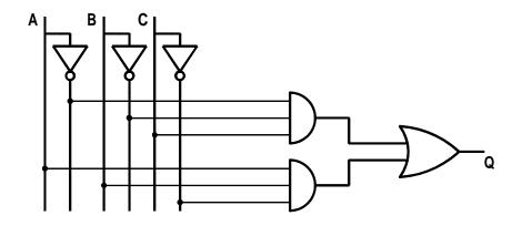
Truth table for  $Q = \overline{AB}C + AB\overline{C}$  and the Sum of Products circuit.
