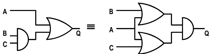
Logic circuit for Postulate 2;  $A + (B.C) = (A + B).(A + C)$ .
