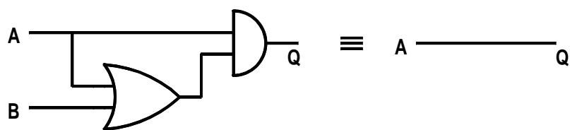
Logic gate circuit representing Theorem 3b;
