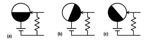
Measure the angle of a shaft by using a set of brush contacts and a segmented metal disk
