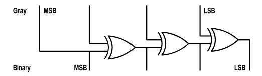
A circuit for converting a four bit Gray code to a 4 bit Binary code.
